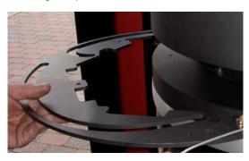
Be careful not to loose this bushing, when the guide plate is dismounted.
