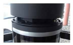
Dismount three screws and bushings in order to remove the guide plate for the door. Be careful with the bushing in which the screw is fastened underneath the guide plate – this bushing is loose (see picture # 6).
