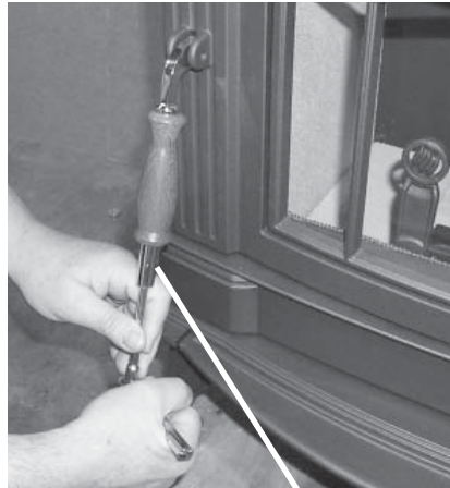
Secure using 7/16" socket wrench.
